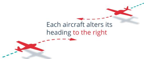
Where an aircraft is required to give way to another aircraft, the aircraft must not be flown so that it passes ahead, or directly over, or under the other aircraft so closely that there is a collision risk.
