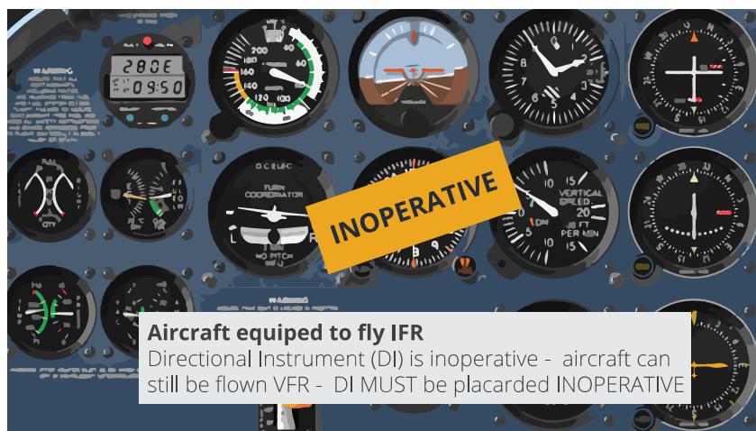
Figure: Example of an inoperative placard
