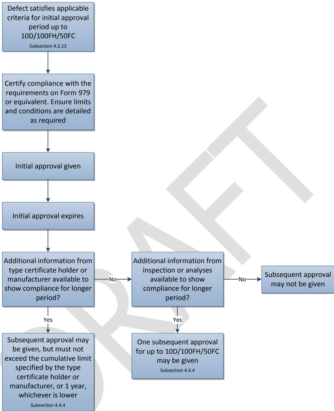
Figure 7: Approval process with 10D/100FH/50FC limit
