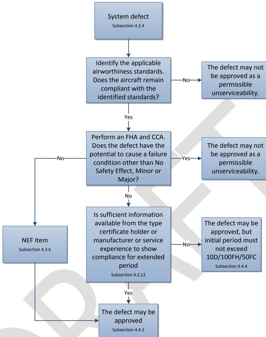
Figure 4: Assessment process for system defects
