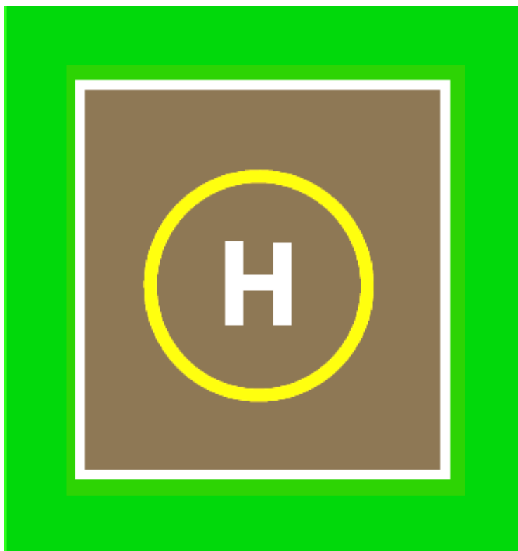
Figure 1: Standard HLS – A 1 \times D TLOF within a 1.5 \times D FATO and additional 0.25 \times D Safety Area (Total area is 2 \times D ). Also showing 'H', FATO perimeter and TD/PM markings.
