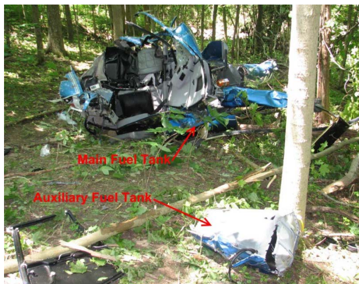
Images highlighting how the RHC SB 78 bladder fuel tank modification, survived the impact forces, and the absence of post-crash fire.
