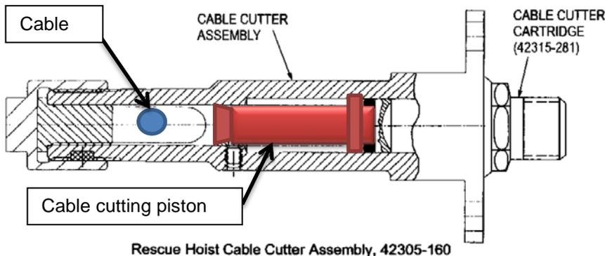
*The squib or cartridge is a pyrotechnic device where a small amount of electrical energy is used to liberate a large amount of chemical energy (an explosion) which powers the cable cutter or guillotine.*
