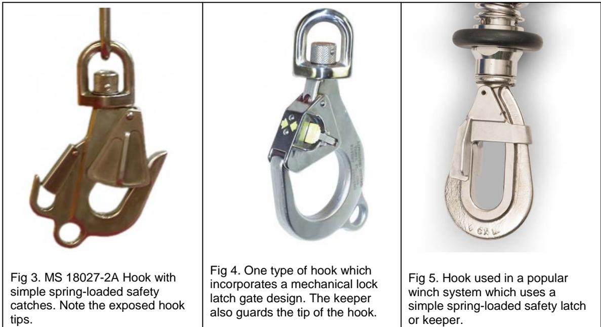
Whenever the personnel harness ring moves up and over the tip of the hook and rests on the simple spring-loaded keeper or guard, the ring will open the guard and slip off the hook when the load is re-applied. Dynamic-rollout or ring reversal is prone to occur with hooks which only have a simple spring-loaded keeper or guard and no mechanical keeper locking mechanism.
