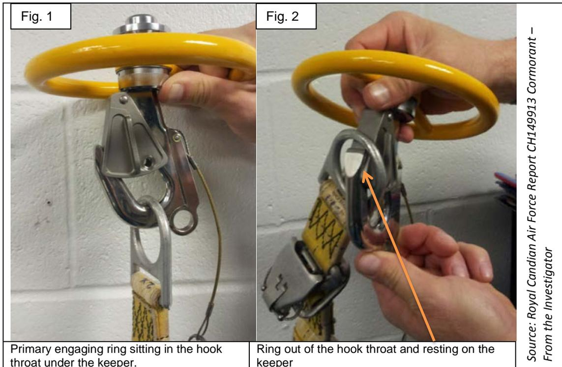
When the winching sequence commences, the load is re-applied, and the ring opens the spring-loaded safety catch slips off the hook and the occupant or load falls to the ground.
