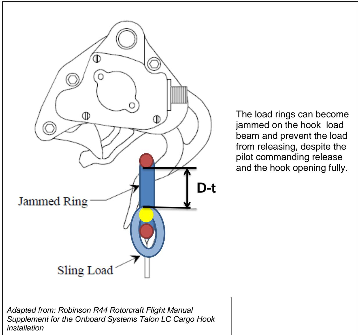
**Fig 3.** Load does not release from an open hook.
