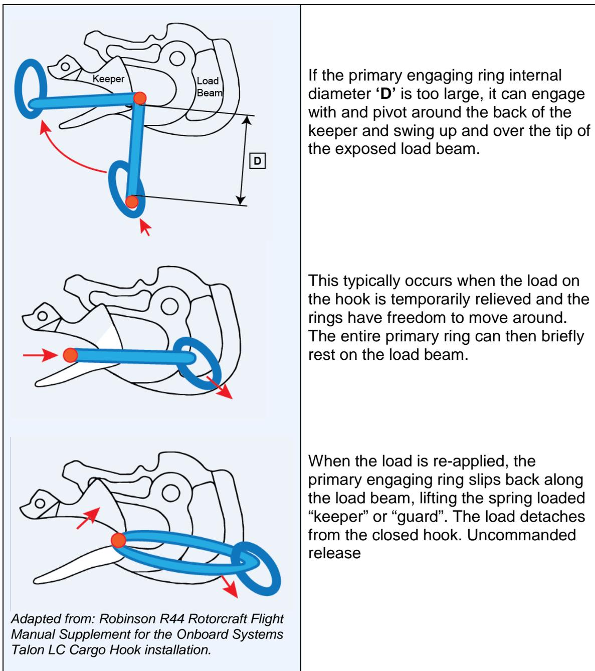
**Fig.2.** Classic cargo hook dynamic roll-out / ring reversal sequence.
