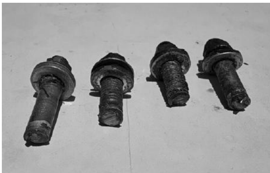
Figure 3. The four missing mounting studs were found on ground, close to the landing site
