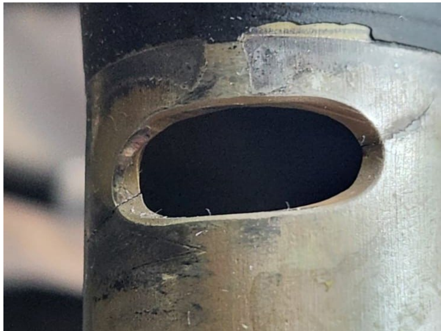
Figure 2. Crack presentation of the first finding reported to CASA.
