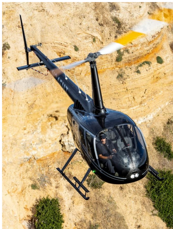
Figure 3 – A Robinson R66 with symmetrical stabilizer
