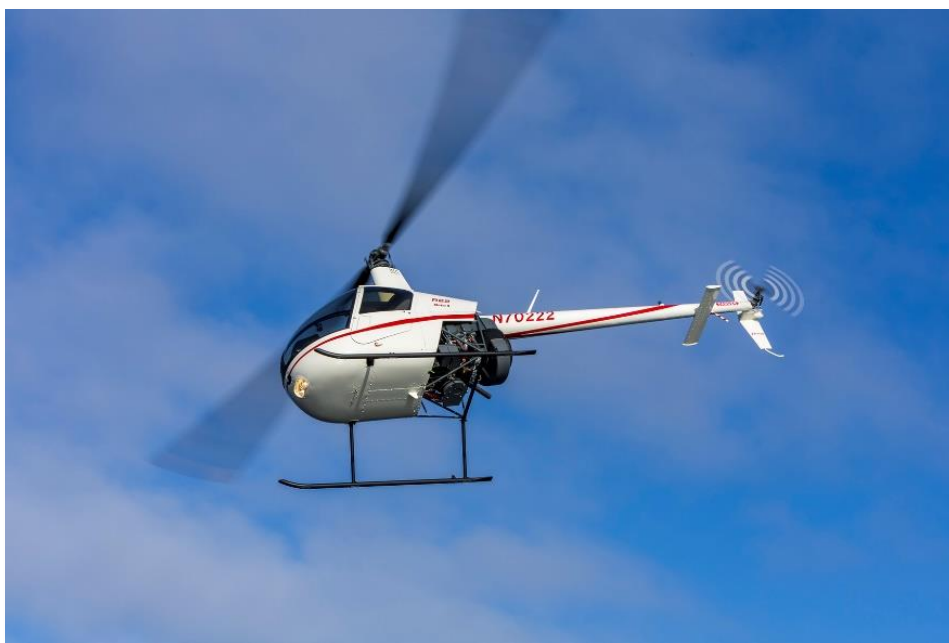
Figure 1 – A Robinson R22 with symmetrical stabilizer
