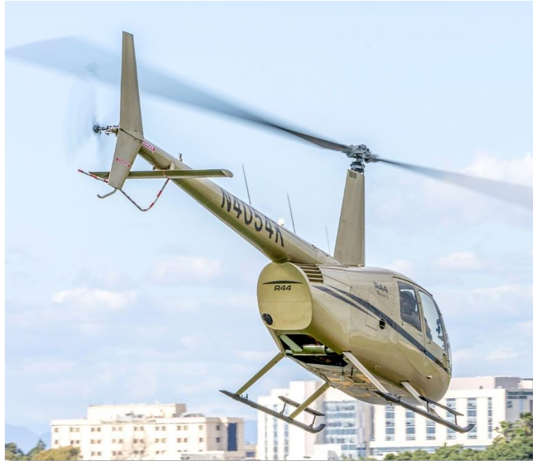
Figure 2 – A Robinson R44 with symmetrical stabilizer
