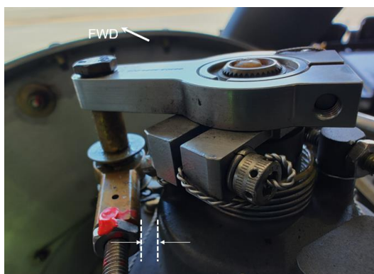
Figure 6. Nil contact between the cable (including the rod end) and the governor body.
