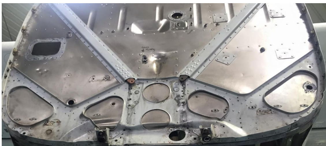
Figure 2. Engine firewall openings that may be opened for maintenance and repairs.
