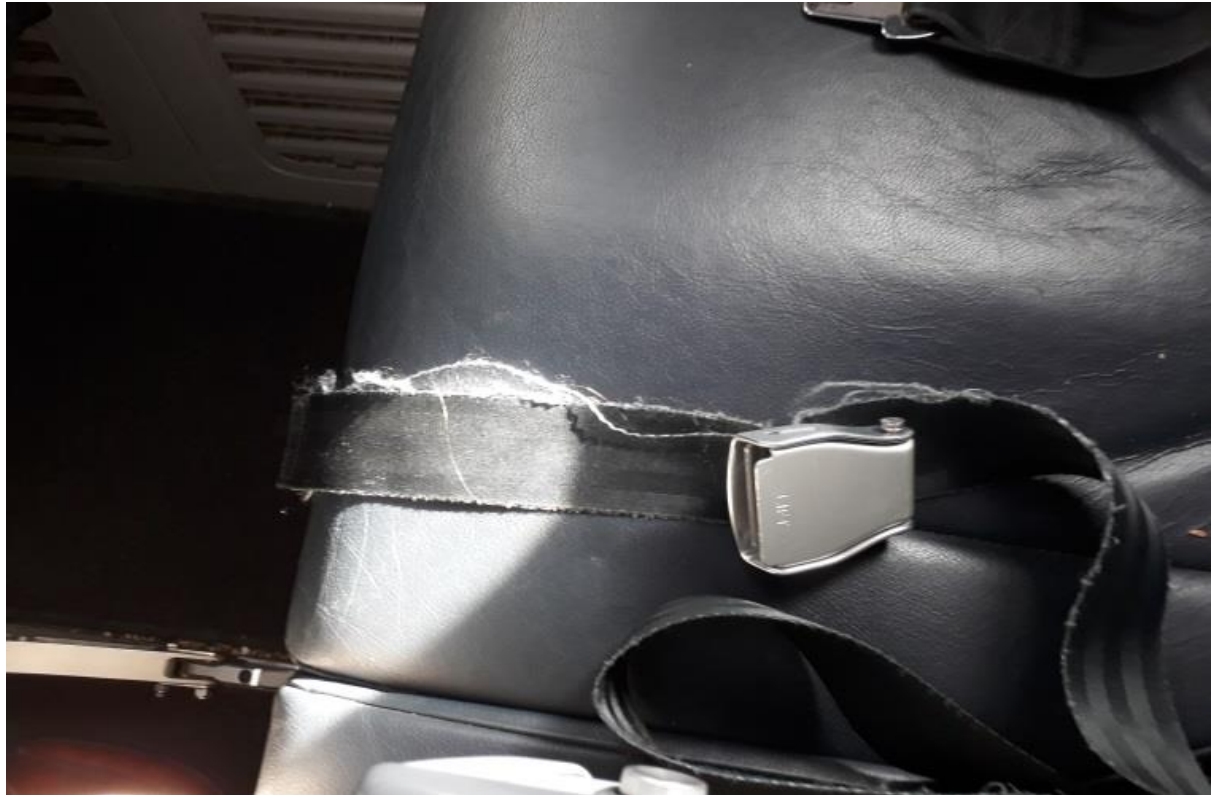
Frayed passenger seatbelt. Source: CASA
