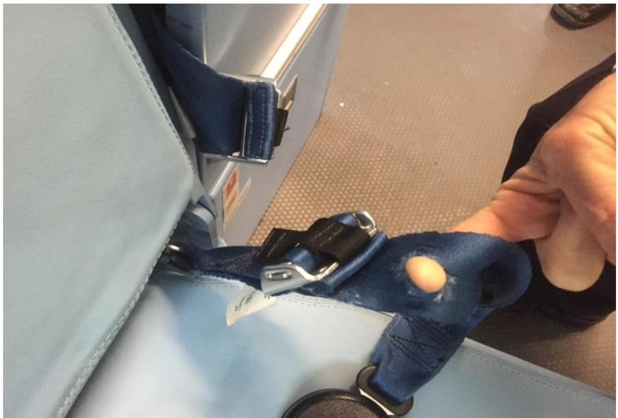
Damaged crew harness. Source: CASA
