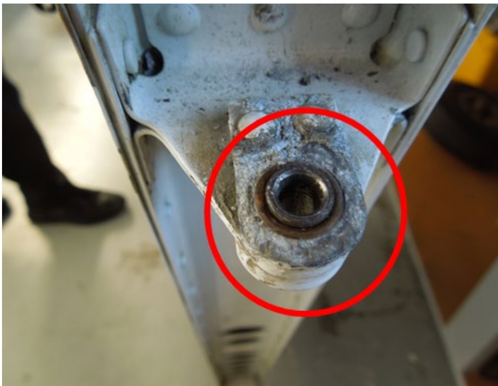
Figure 1. Centre Rudder Hinge Mount Corrosion
