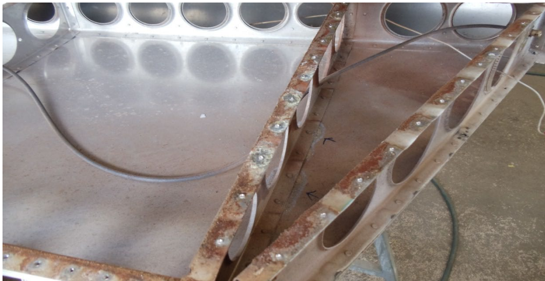
Figure 4. Cessna 152 vertical fin corrosion
