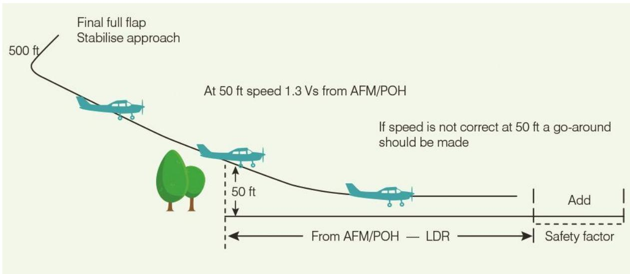
**Figure 5: Landing distance with additional safety factor**
