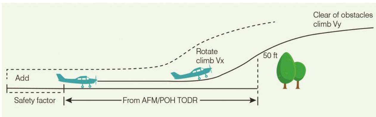
**Figure 4: Take-off distance with additional safety factor**
