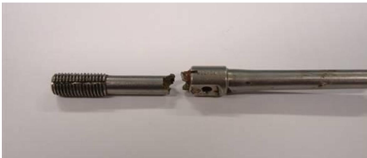
Figure 1 - Flight control cable terminal separation
