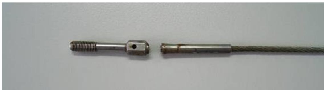
Figure 2 - Flight control cable terminal separation.
