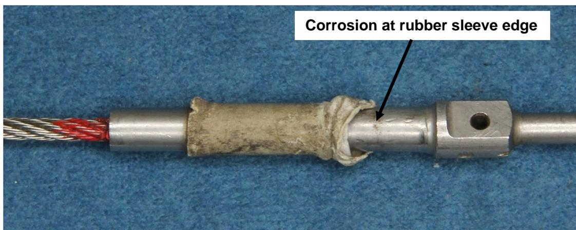
Figure 4 - Control cable terminal section covered in rubber sleeve
