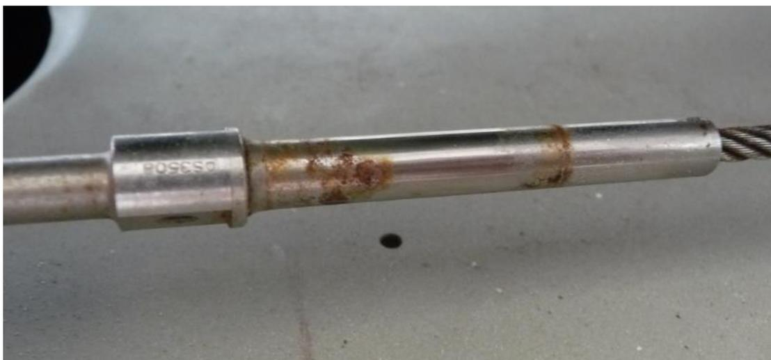
Figure 6. Source: CASA SDR. One of the eleven corroded primary flight control cables on the single aircraft. Corrosion originated from under the rubber sleeve.
