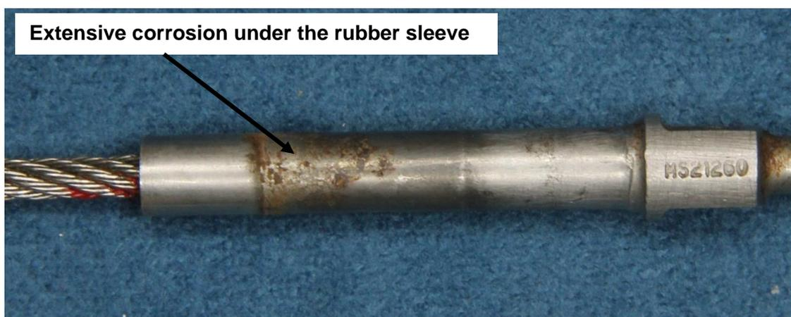
Figure 5 - Control cable terminal shown in figure 5, with the rubber sleeve removed. Note extensive corrosion. (Source: ATSB Investigation AE-2012-028 Final – 9 April 2013).
