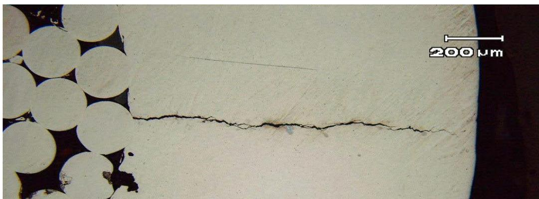
Figure 7 - Internal corrosion - flight control terminal sleeve.
