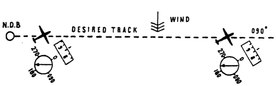
Figure 8: Backtracking (that is, Allowance for Drift)
