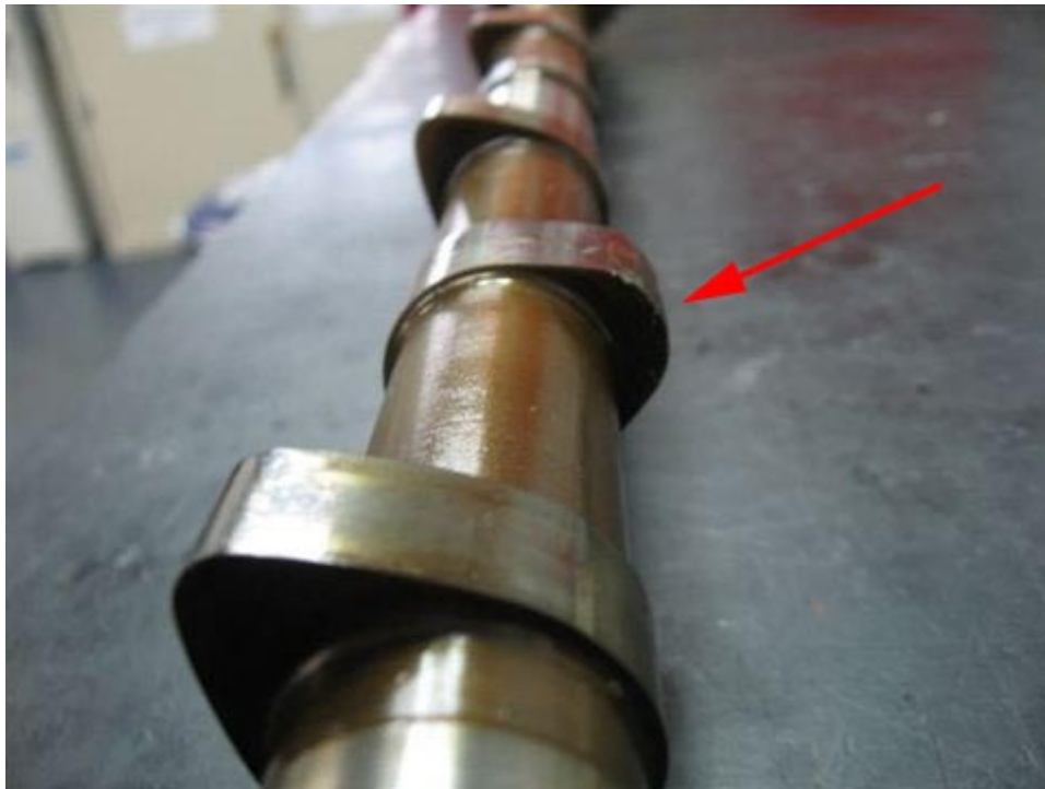
Figure 5 - Worn Lycoming camshaft lobe which was operating with a spalled tappet body P/N15B26064.
