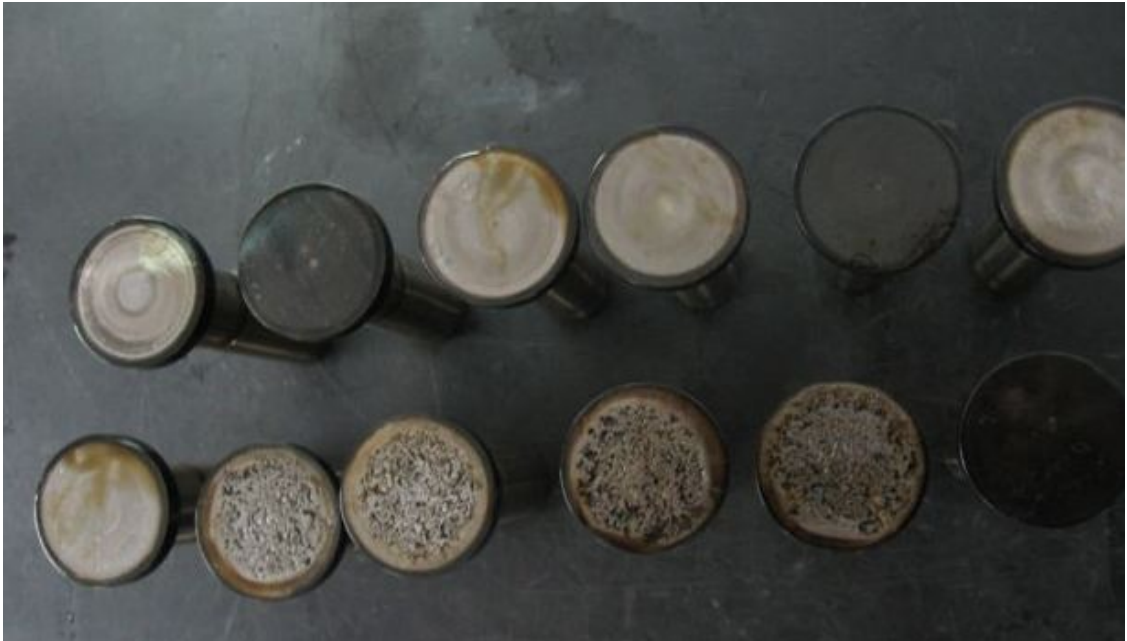
Figure 2 - Spalled P/N 15B26064 tappets showing the various stages of deterioration that can exist between tappet bodies in one engine.
