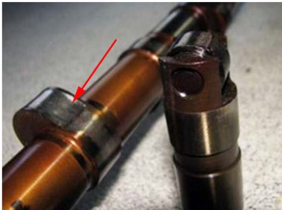
Figure 6 - Lycoming roller cam follower and worn cam lobe.
