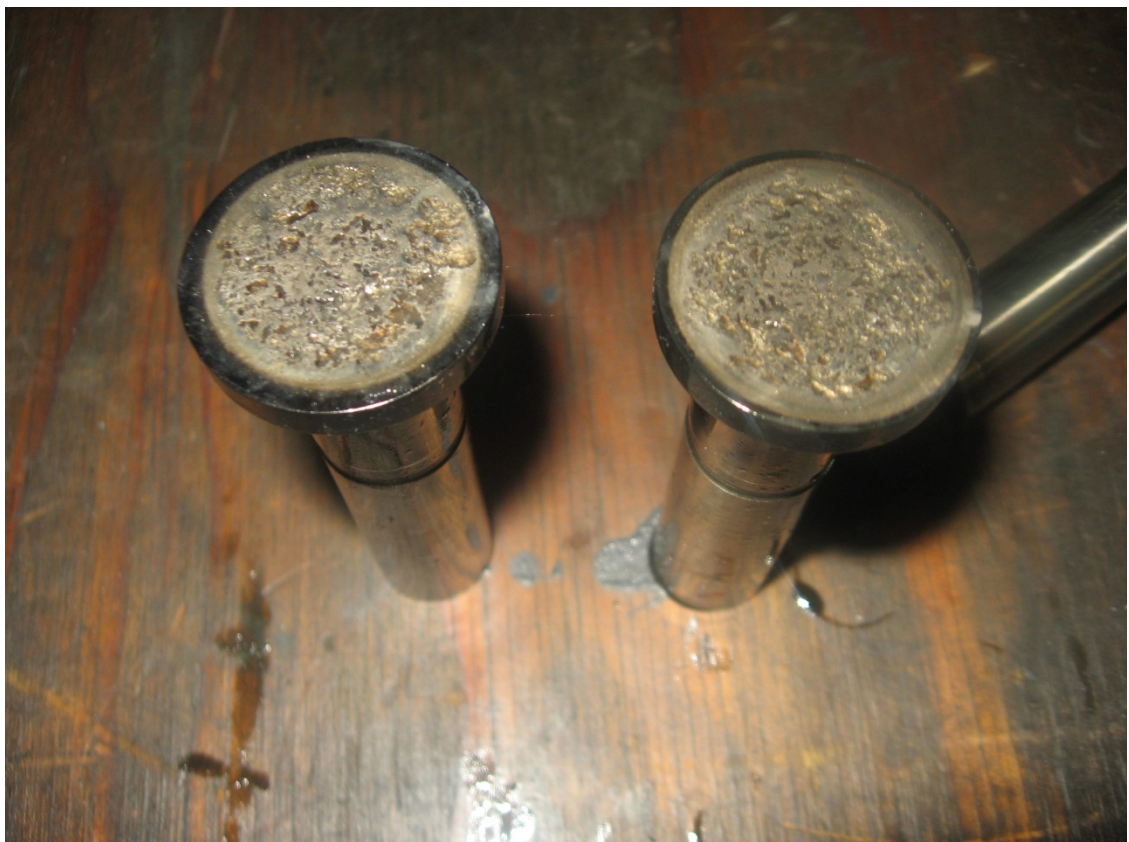
Figure 1 - Advanced spalling of Lycoming tappet body P/N 15B26064.
