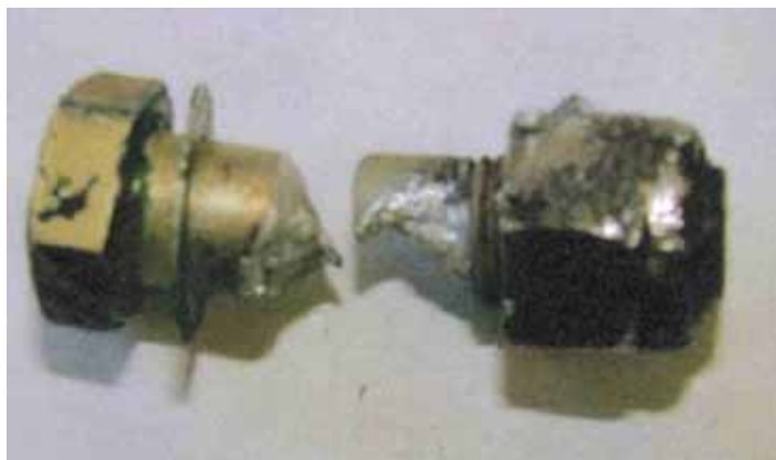
Figure 2: Corroded Earth Terminal Point
