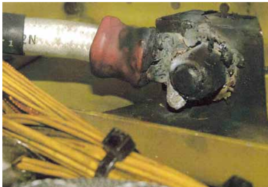
Figure 1: Corroded and burnt Earth Terminal
