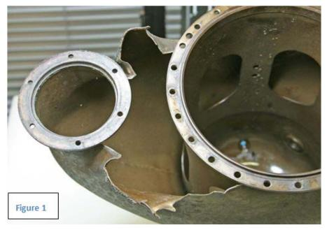
Figure 1. RR 250 C47B OCC Rupture failure (RH Side) Source: ATSB AO-2008-067.
