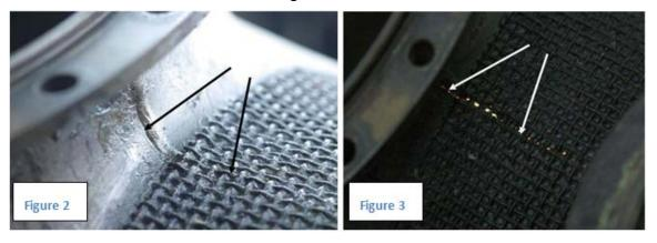
Figures 2 and 3 Depict RR 250 C47B OCC (LH side) showing two views of cracking in the same OCC duct shown in Figure 1. Fig 2 shows external indications, Figure 3 the same crack viewed with a strong light placed inside the OCC. (Source: ATSB AO-2008-067)
