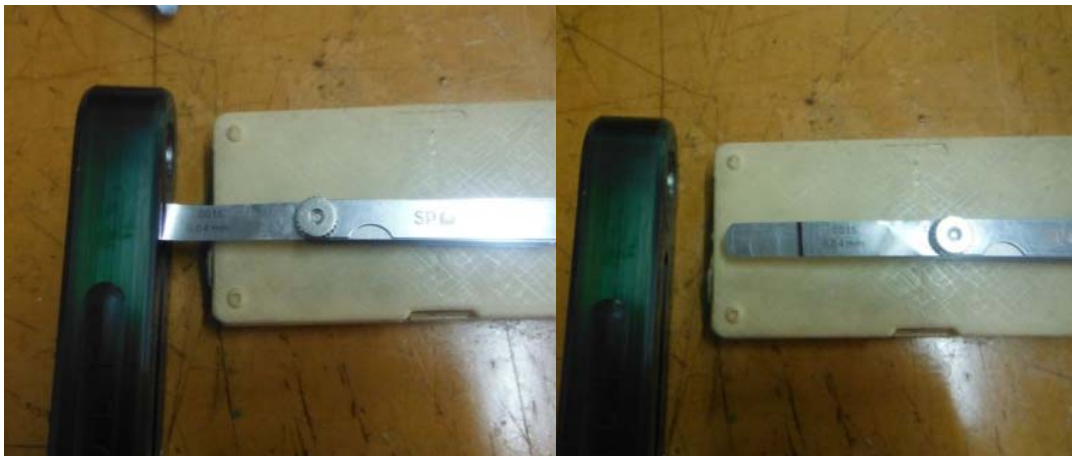
Fig. 1a and 1b Showing penetration of a .015" Feeler gauge in the urethane casing of an Airwolf TT strap.
