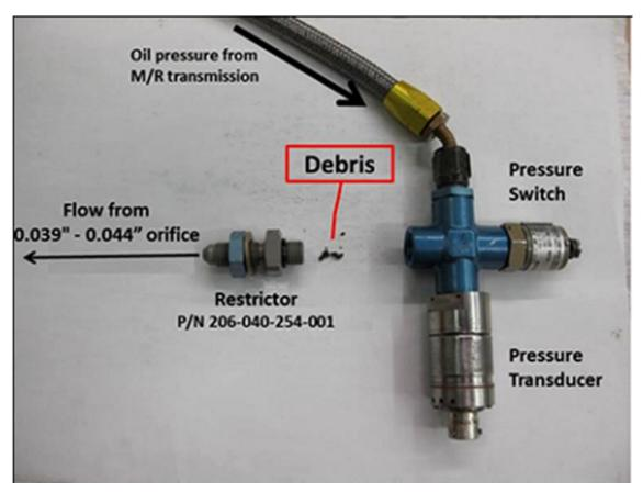
Fig. 2 - General arrangement of the failed freewheel oil supply, also note the debris blocking the restrictor or oil jet. (Ref. TSB Aviation Investigation Report A11C0152).
