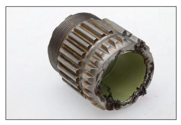
Fig. 3 - Upper mast stub which separated from the main rotor mast. (Ref. TSB Aviation Investigation Report A11C0152).
