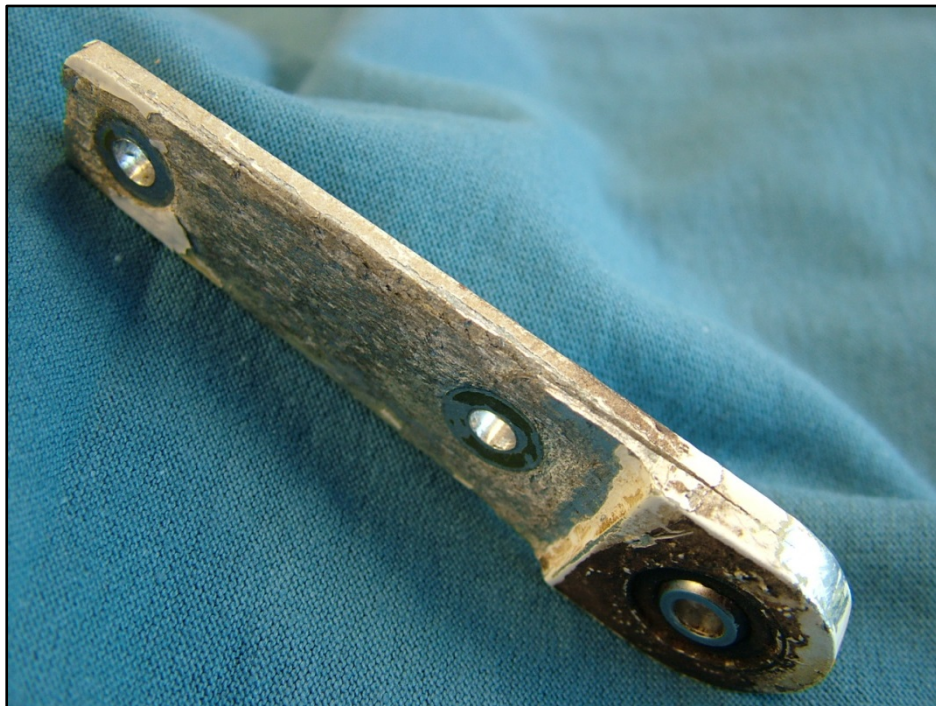
Figure 1 Corroded Aileron Hinge
