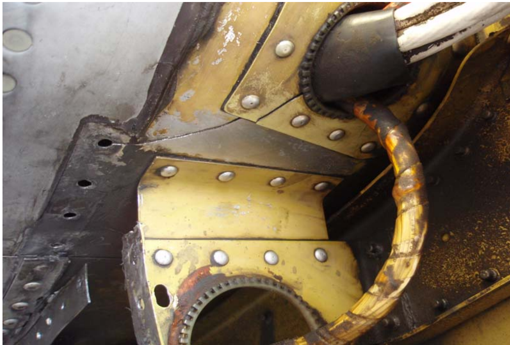
Photo showing approx 4 inch crack at Station 81. View from inside leading edge. Note crack has been arrested by a fastener hole. Cracks in the skin may be visible externally.
