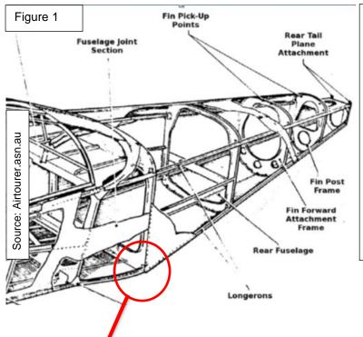
Corrosion in these longerons severely reduces the structural integrity of the aircraft, which is certificated for a wide range of aerobatic manoeuvres.
