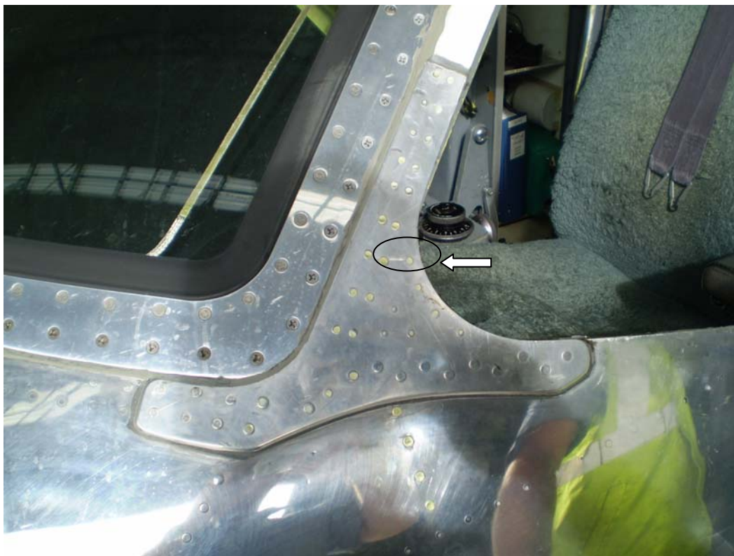
Figure 2 – showing external doubler installed. Initial crack has originated from the edge of the doubler to a low edge margin fastener at a location indicated by arrow in the figure. The crack has propagated between the group of three fasteners (circled).
