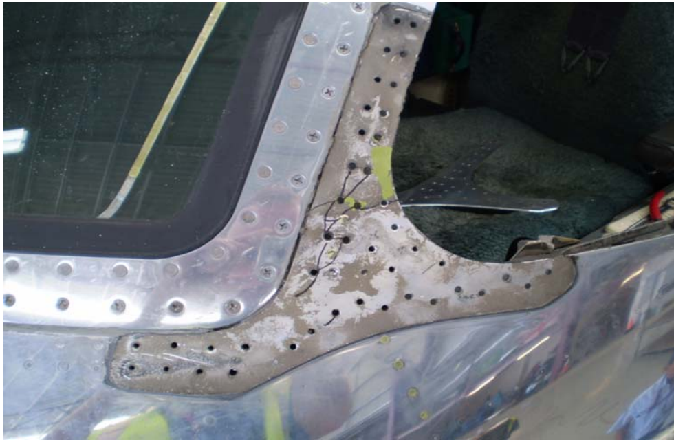
Figure 1 – Underlying fuselage skin cracking. This cracking would be hidden from view by the overlying external doubler which is installed IAW SB120-53-0072. Figure 2 shows the external doubler installed.
