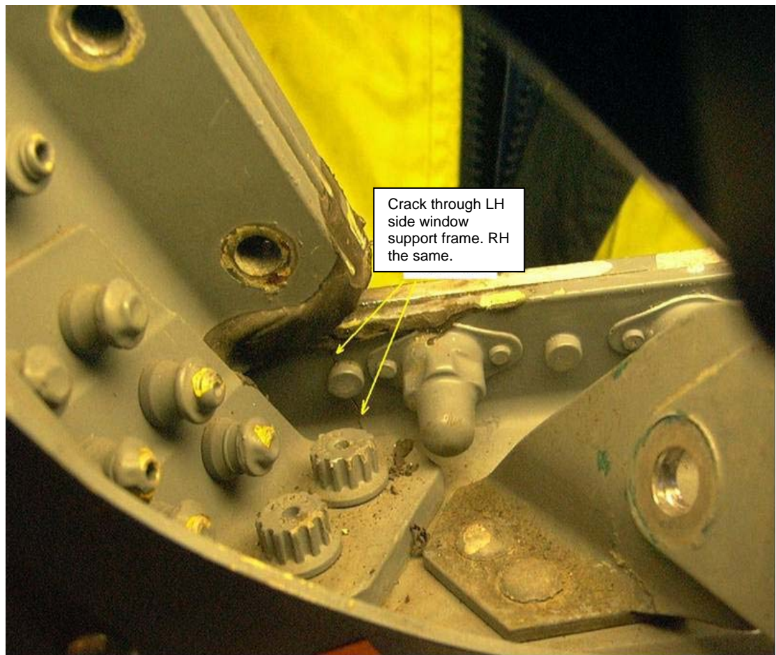
Figure 3: Cockpit window lower support frame cracked from rivets on LH and RH sides.
