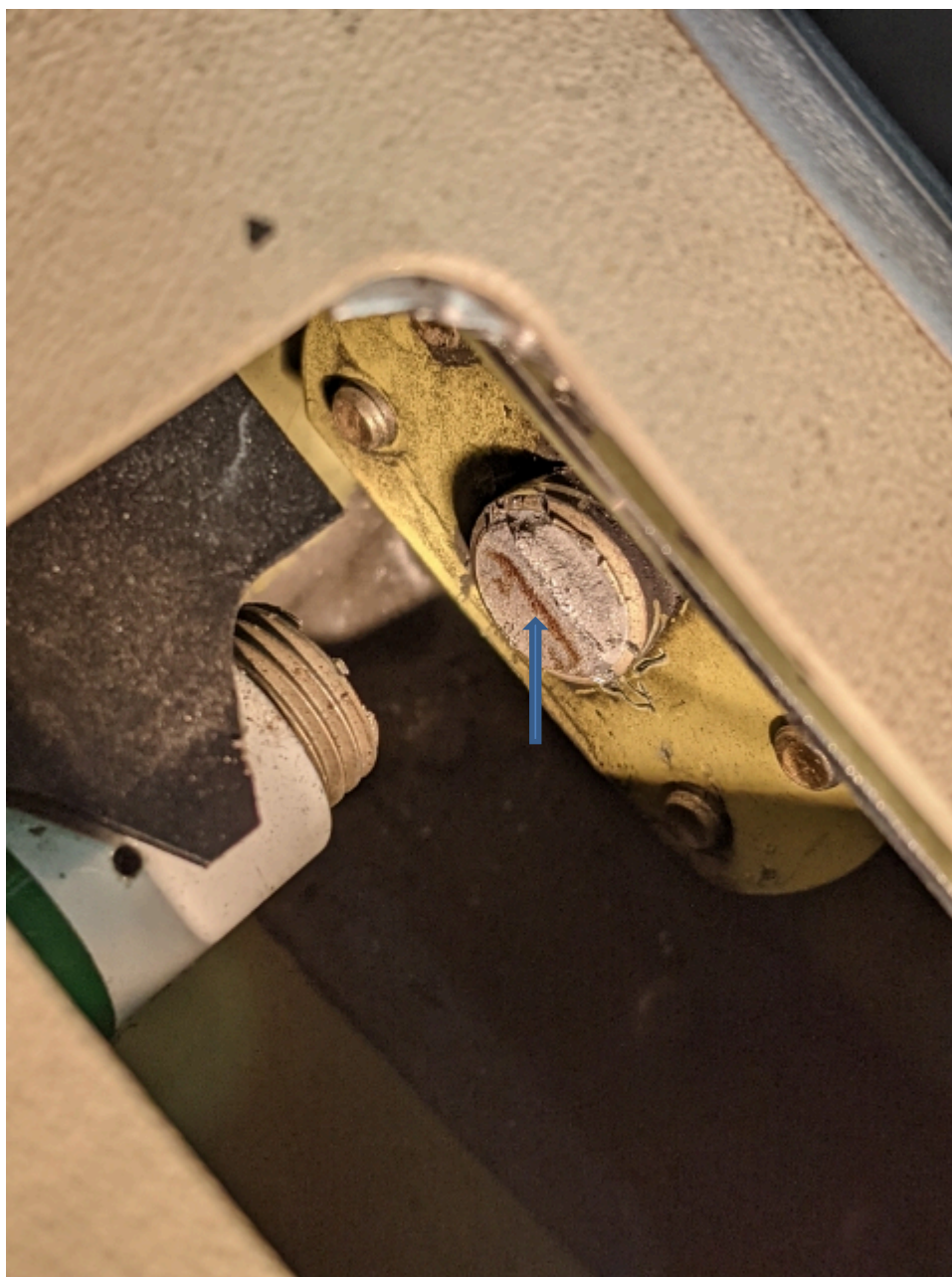
Figure 2: Closer view showing fracture of threaded area. Arrow indicates corrosion product which indicates the crack was present for some time.
