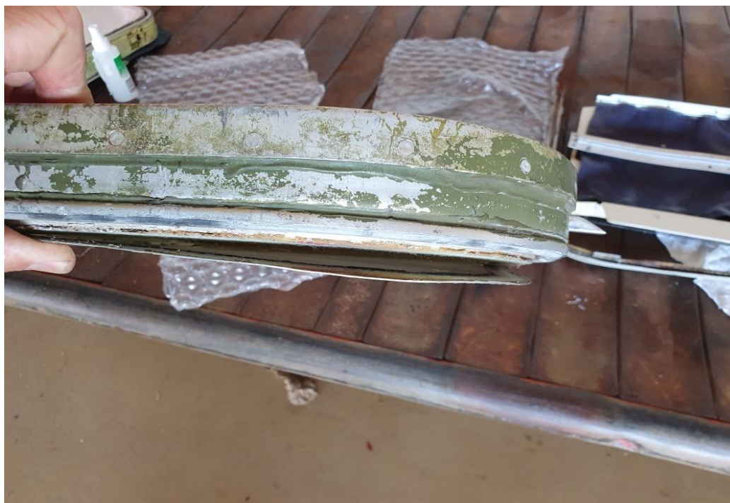
Figure 5: View of external edge of door showing skin lifted after disbond
