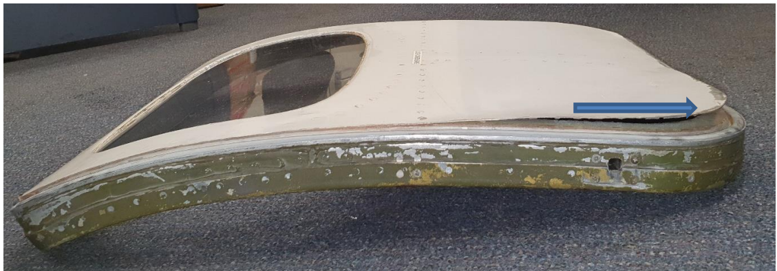
Figure 1: Lifted edge of skin after disbond
