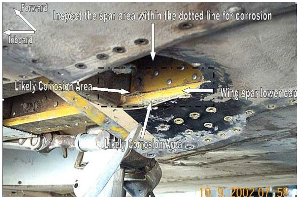
Figure 1: Inspection Area - Left wing with inspection access panel number 12 removed.
