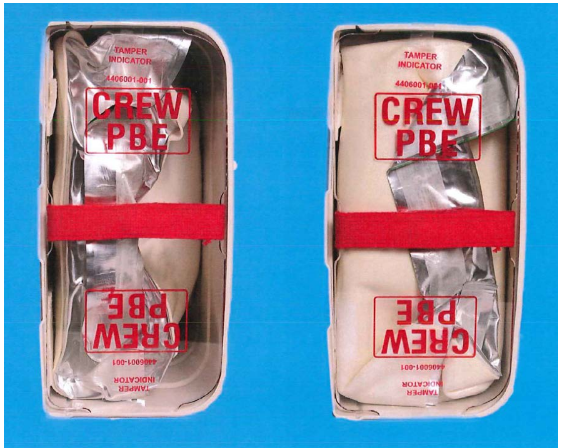
Condensed Pouch Indicates Intact Seal
