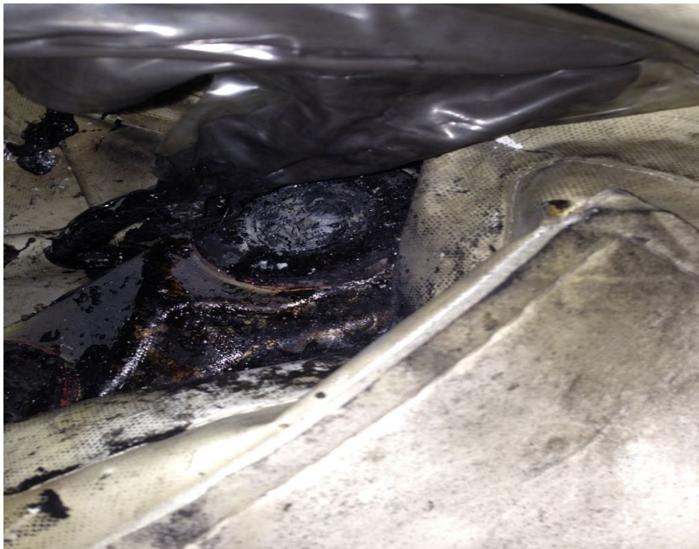
Figure 9 – Soot from exploded canister
