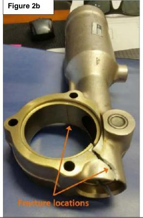
There have been other cases of Cessna single engine retractable aircraft where the main landing gear could not be either fully retracted or extended due to broken actuator piston rack teeth, or due to the housing cracking open, resulting in actuator disengagement.
