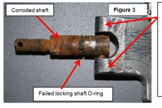
Note the corroded shaft and worn latch handle bearing plates (or cams).
