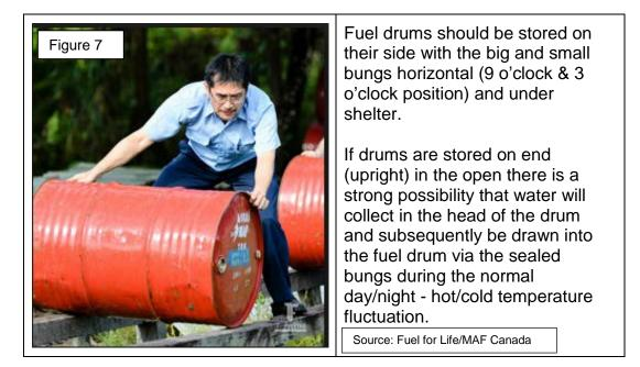
Reject fuel from any drum if the seals are broken, or if the fuel is past the displayed expiry date. Aviation fuels have a comparatively short storage life. Using fuel past the expiry date may result in unpredictable engine performance.
