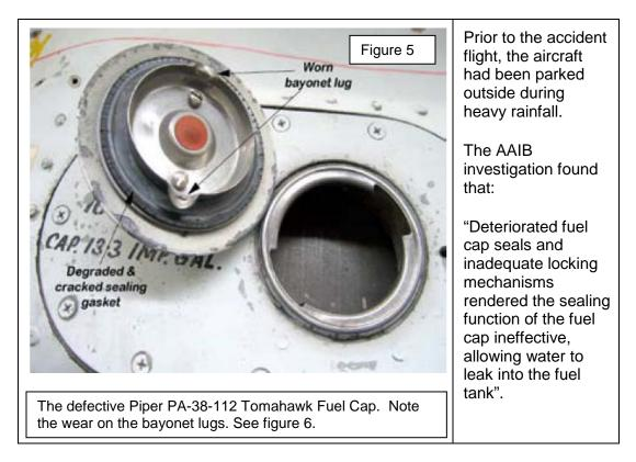
This design relies on two very thin and stiff circumferential springs behind the thin seal to ensure the two locking tabs in the cap remain firmly engaged in the locking detents in the tank and pressure is maintained on the seal when the cap is closed. The bayonet lugs were badly worn and the seal badly degraded.
