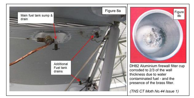
Water from the fuel system collects in the aircraft main fuel sump or gascolator which is typically made of aluminium or cadmium plated steel, and prone to corrosion, particularly in the presence of standing water. (Figure 8b) This is another reason for fuel filter gascolators/sumps to be drained, cleaned and inspected at the calendar interval as well as at the periodic inspection interval.
