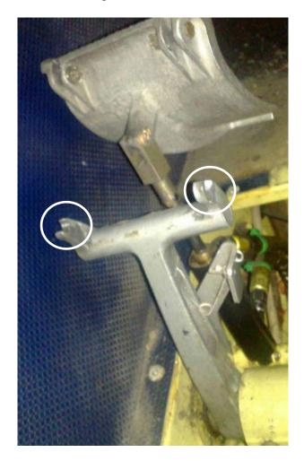
Figure 1: Rudder pedal arm with failed brake pedal pivot holes
