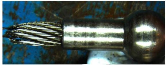
Image courtesy of ATSB Figure 3. Swaged (Ball) end of failed cable
