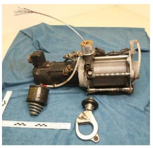
Image courtesy of ATSB Figure 1. Failed Hoist Assembly (Winch, Bumper and Hook)
