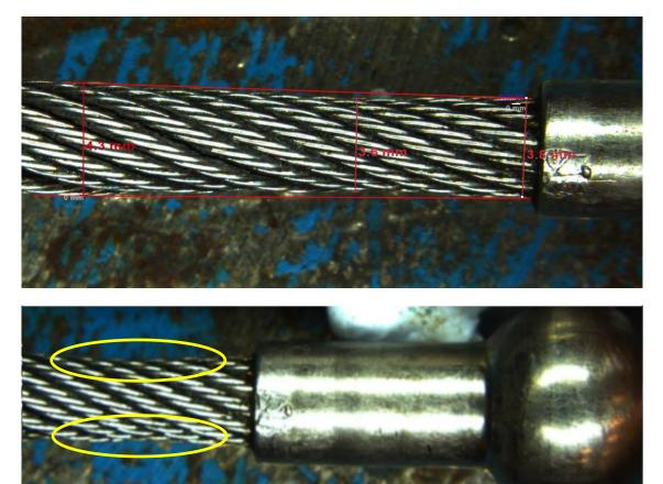
Image courtesy of ATSB Figure 8. Operational cable with local necking and measurements
