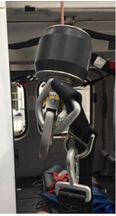
Figure 1 - Ring reversal with ring and webbing about to activate the dual lock latch gate
