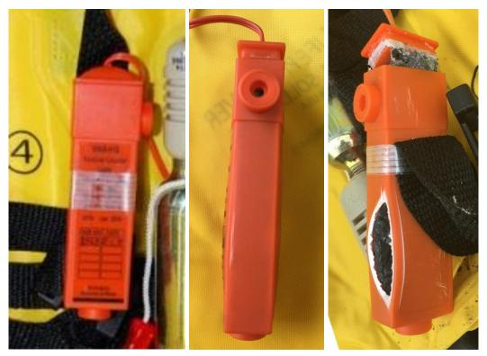
Figure 1: Left to right – Serviceable battery, unserviceable battery (note swelling of main body and endcap pushing off), failed battery.
