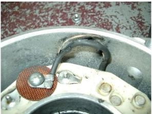
Figure 6 - Diode block wiring short circuit
