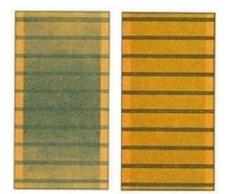
Figure 5 - Out of round compared to good condition commutator
