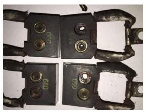
Figure 8 - Loose starter/generator brush rivets
