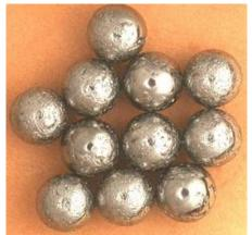
Figure 3 – Spalling damage
