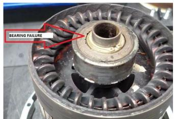
Figure 4 - Bearing failure
