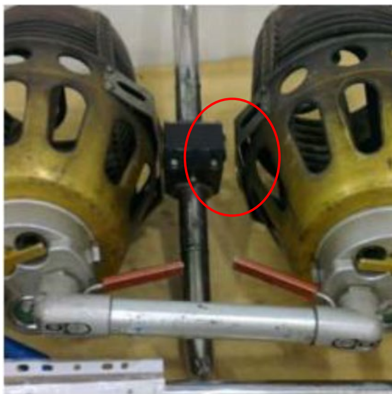
Figure 1: Double Stratus Burner Unit (Note: Failed hanger circled in red) Photo Reference: Cameron Balloons SB 28 Rev 0
