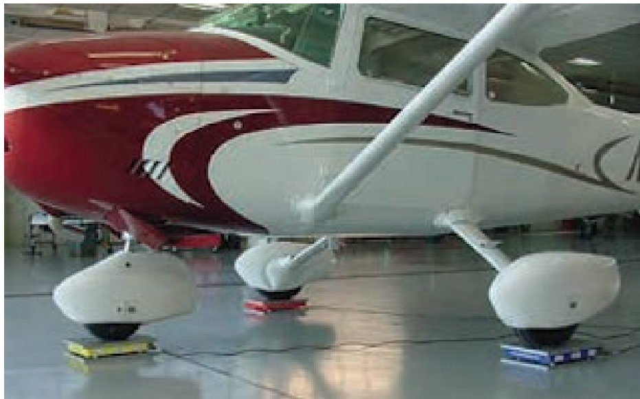
Figure 2. A Cessna 182 being weighed with electronic platform scales
