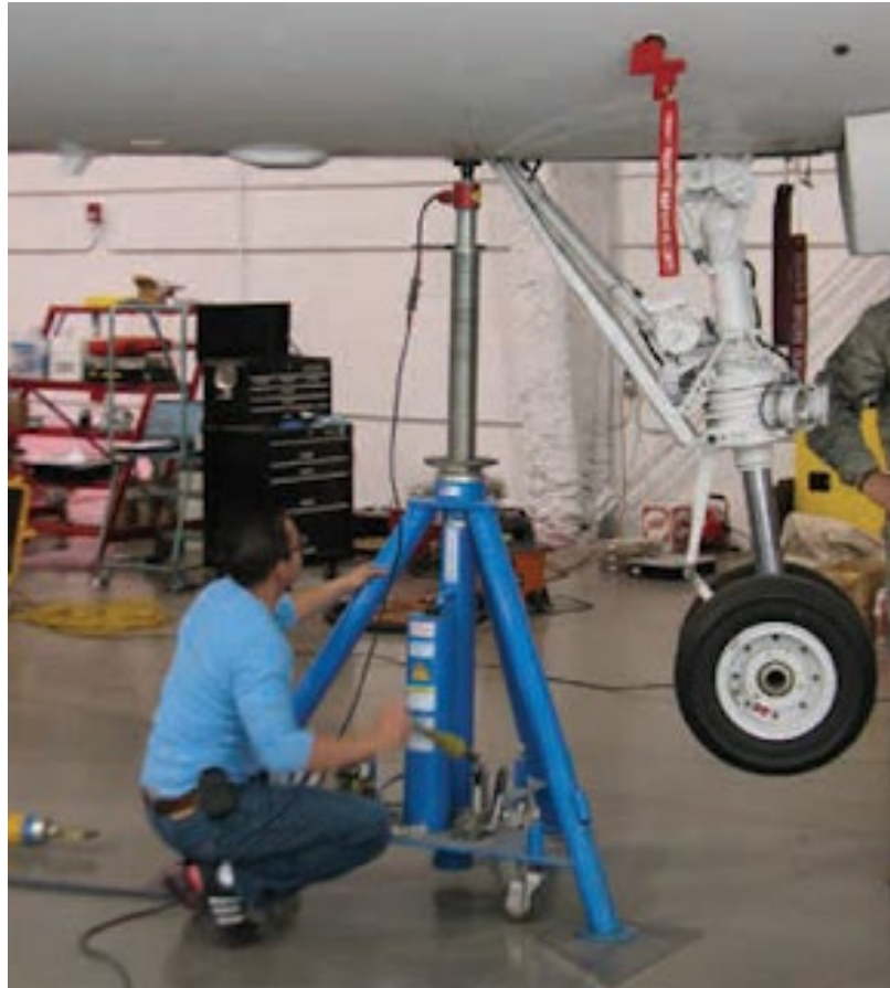
Figure 1. Airplane on jacks with load cell units in use
