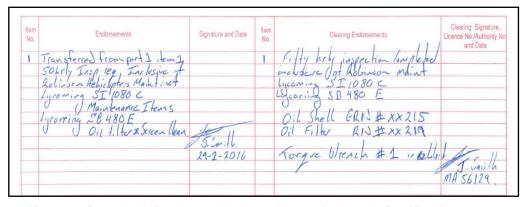
Figure 1. Sample Maintenance Release Part 2, 50 hourly Certification
