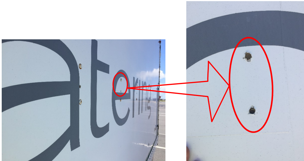
Figure 11. Wasp nest in catering truck panel holes
