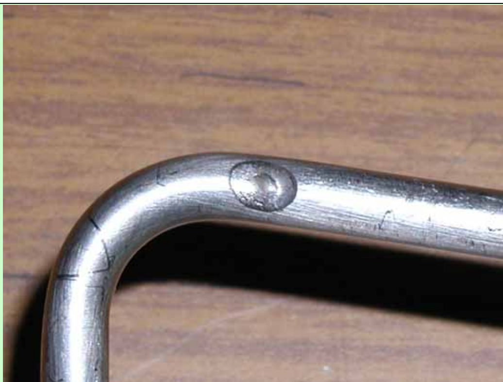
Figure 3 - Tube Assembly - Chafing
