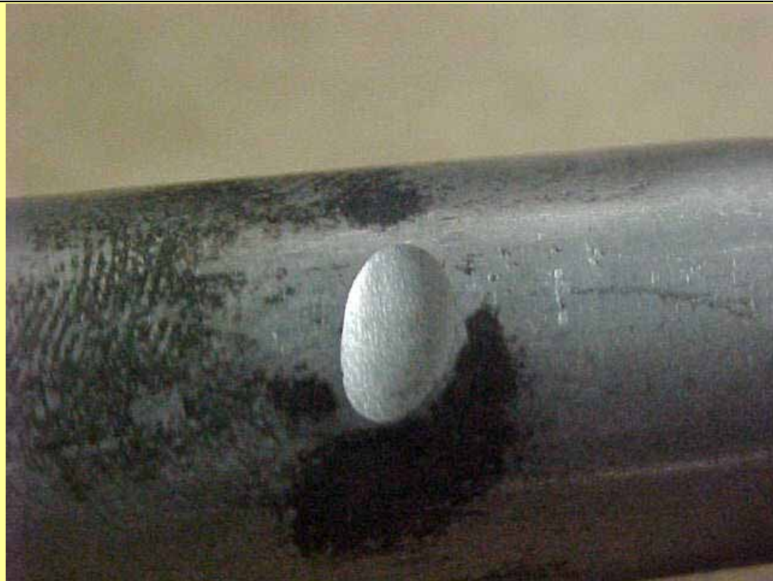
Figure 1 - Tube Assembly - chafing marks and signs of corrosion
