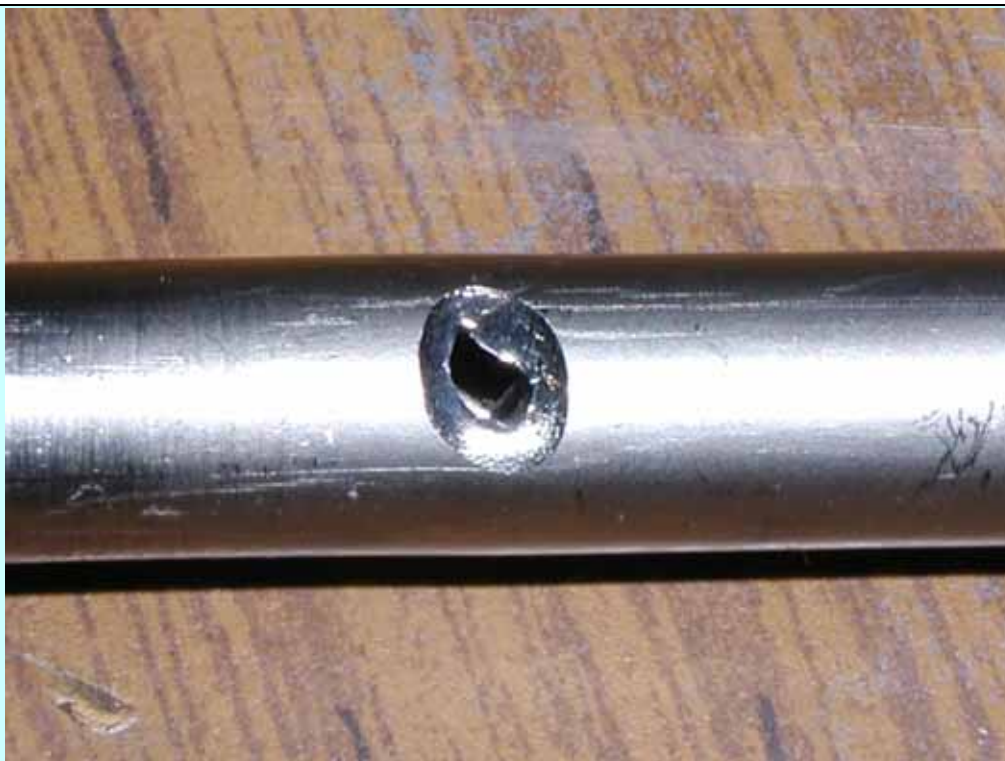
Figure 2 - Tube Assembly - chafing led to holing and fluid leakage
