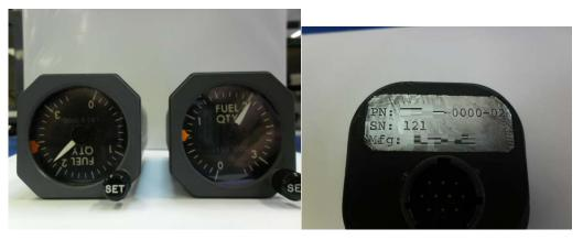
Data plates should clearly identify the manufacturer and type of indicator.
