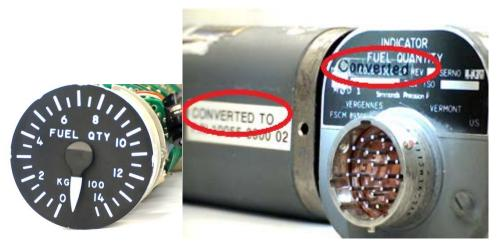
The indicator was received with the previous repairers' tamper–proof seal still intact. This type of inaccuracy could cause a fuel load mismanagement problem.
