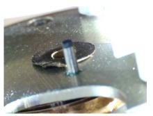
The example above shows a bushing installed instead of a ball bearing. This could lead to premature failure of the indicator and possible loss of indication during flight.
