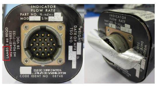
In this example the original data plate can be seen underneath the non OEM approved data plate. Only one data plate should be installed on the indicator. The data plate also states that 2 "LAMBS" are required with their associated part numbers.
