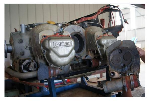
Figure 1. Typical cylinder head separation for Lycoming and TCM engines for illustration purposes only. (The failed cylinder depicted was not repaired by Challenger)
