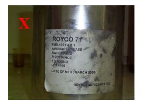
Falsified Label. The type of paper used Lack of trademark Lack of resistance of the label to be affected by the product.
