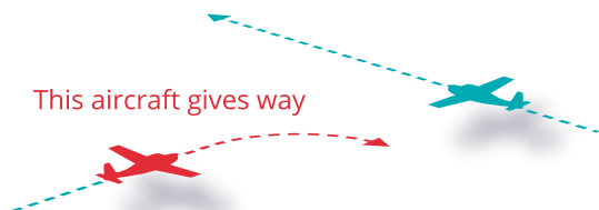
Figure 5: Aircraft with right-of-way to maintain heading and speed
