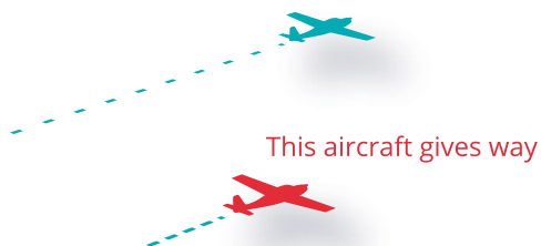
Figure 6: Overtaking aircraft to keep clear and to the right
