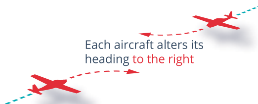
Figure 7: Aircraft approaching head-on to alter heading to the right
