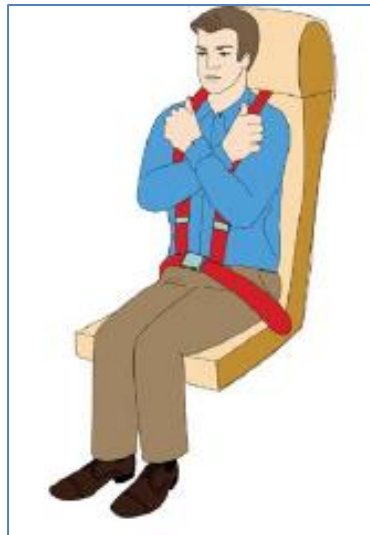
Figure 8: Aft facing seat, lap strap and shoulder harness with dual upper torso straps, onshore helicopter occupant
