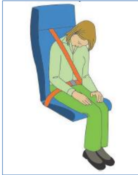
Figure 2: Forward facing passenger seats equipped with a lap strap and shoulder harness with single diagonal strap
