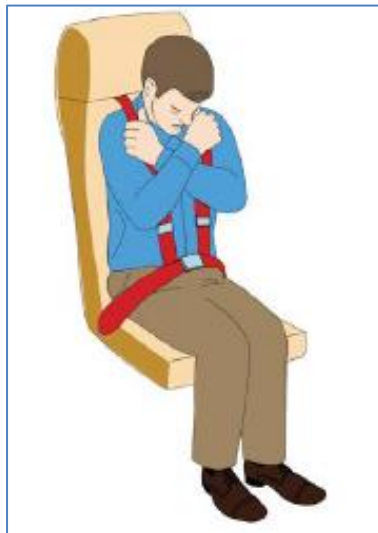
Figure 7: Forward facing seat, lap strap and shoulder harness with dual upper torso straps, onshore helicopter occupant
