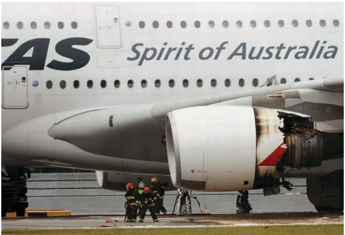
Image: Significant structural damage to the number 2 engine | EPA/STR
