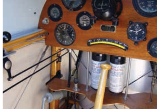
Figure 5 Example of basic flight instruments. Note the joystick that resembles a baseball bat
