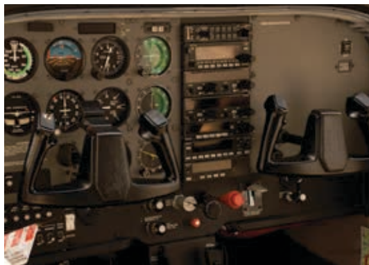
Figure 7 Traditional light aircraft cockpit with enlarged view of the 'six pack' of flight instruments
