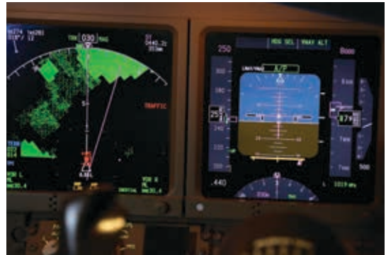
Figure 10 Example of glass cockpit flight displays showing PFD and multi-function display (MFD)
