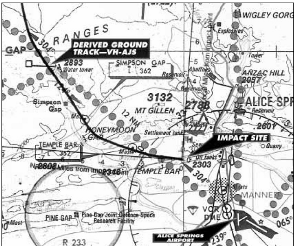
image: plan view showing the track of VHS-AJS during the approach | ATSB Investigation report 9501246
